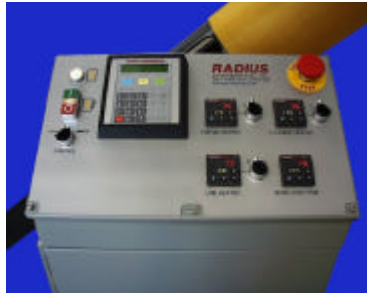
Enclosure control panel for operator interface in "Stand Alone" mode
