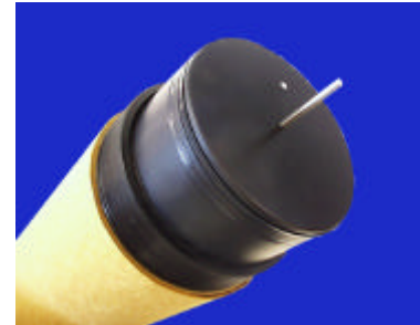
In piston pressure transducer and over-temperature thermocouple for monitoring injection process
